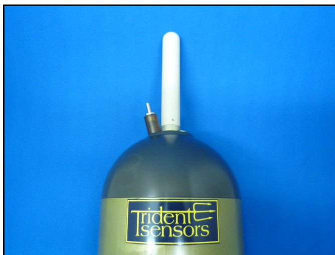
Dual Element Active GPS & Passive Iridium Mounted Directly onto Pressure Housing
